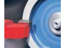
**Resin bonded grinding wheels**
