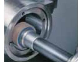
**Resin bonded grinding wheels**
