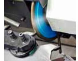
Resin bonded grinding wheels
