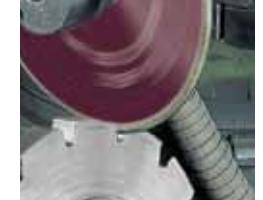
**Resin bonded grinding wheels**
