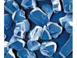
The size of the abrasive grits determines the effect of grinding and the quality of the grinding surface.
