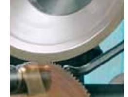
Resin bonded grinding wheels
