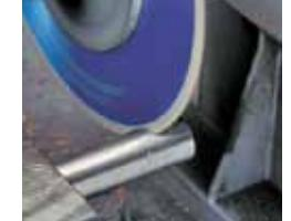
Resin bonded grinding wheels
